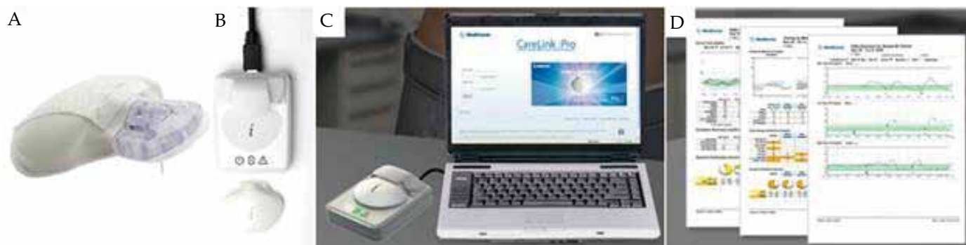
Fig. 1: Components of the iPro2 System. Panel A shows the iPro2 recorder attached to a subcutaneous glucose sensor (the small filament protruding from the bottom right). Panel B shows the iPro2 Smart Dock (top) and the iPro2 recorder (bottom). Panel C shows data being uploaded to a remote server from the iPro2 via the Smart Dock. Panel D shows 3 report formats available from an iPro2 study - the Daily Overlay, Overlay by Meal, and Daily Summary
